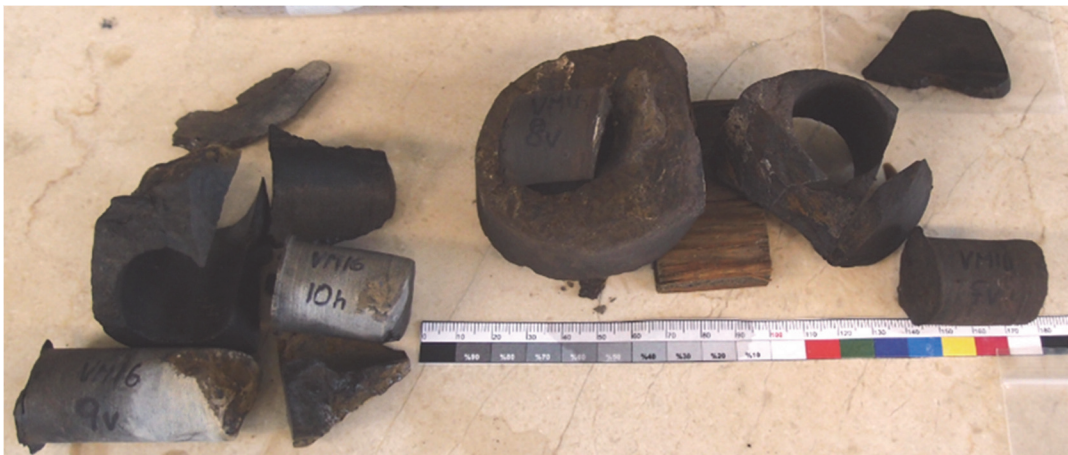
Figure 2. Example of core plug extraction at several different angles at almost the same sampling location.
