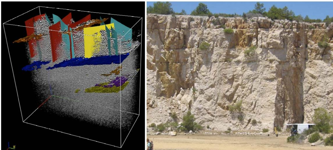
Figure 2: Left: GPR volume (values of minimum amplitude are removed) with stratigraphic and fracture interpretation. The blue horizon acts a mechanical unit boundary against which the large fractures terminate. Right: A major fault offsetting the quarry wall is one of the green faults interpreted in the GPR data. This fault like most fractures strike  $N080^\circ$  and are sub-vertical.
