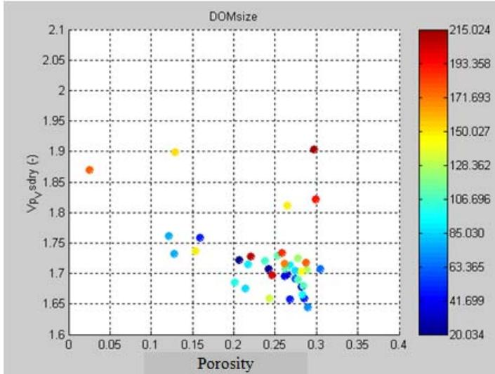
Figure 1: Cross plot of porosity and  $V_p/V_s$  ratio for a sample set of dry measurements from a Middle Eastern limestone reservoir. Superimposed is the digital image analysis parameter Dominant Poresize (in microns). No clear relationship is visible between pores structure data and  $V_p/V_s$  ratio.  $V_p/V_s$  ratio shows a negative correlation with increasing porosity, indicating that  $V_p/V_s$  ratio is non-constant with porosity.
