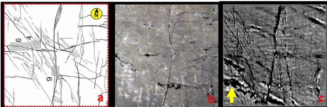
Figure 1: (A) Part of line drawing of deformation bands on the quarry floor by Tondi et al. 2006. (B) Aerial photograph of the same area; 20 m x 20 m wide. (C) Horizontal slice at 40 cm depth through one of the 3D GPR volumes displaying the deformation bands in great detail. The yellow arrow represents the direction of GPR data acquisition.
