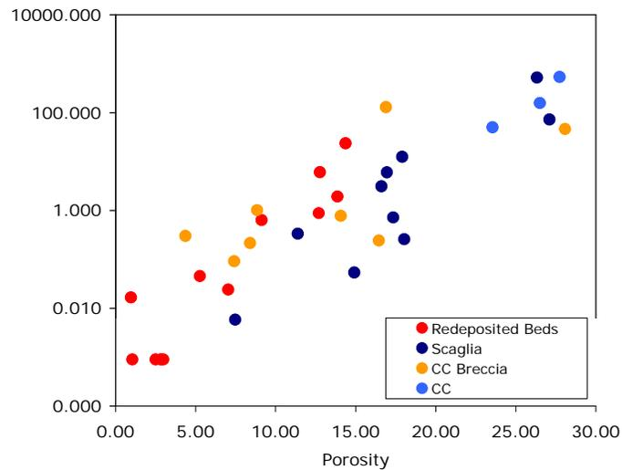
*Figure 1: Porosity versus permeability of megabreccias and turbidites (red dots) and the corresponding background sediment (Scaglia, dark blue dots). Breccias rich in rudist debris (Calcare Cristallini, orange dots) have generally less porosity and permeability than the coarse-grained rudist grainstone (Calcare Cristallini, CC, light blue dots).*
