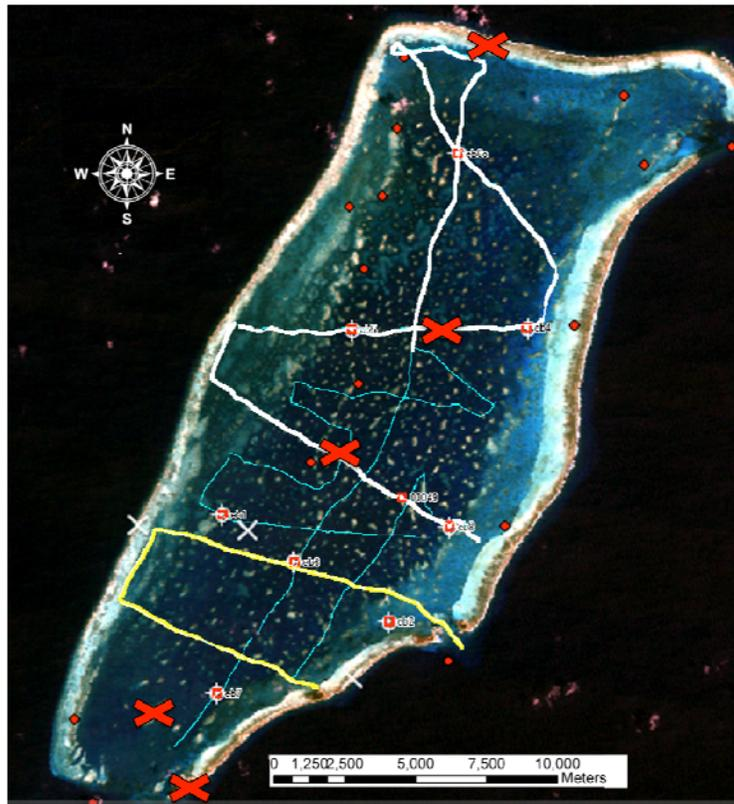
Figure 1: The locations of the potential drill sites are shown as red crosses. White, yellow and blue lines indicate the seismic grid collected in March 2008.
