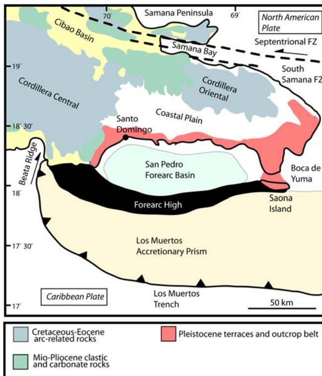
Figure 2: Geologic and tectonic map of southeastern Dominican Republic. The Pleistocene terrace and outcrop belt is shown in red. Modified from Mann et al. (1995).
