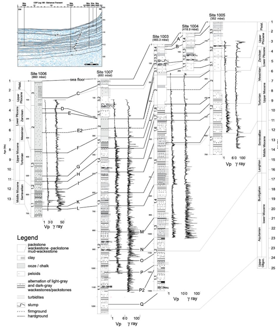
Figure 2: Lithologic, velocity and natural  $\gamma$ -ray log of Neogene carbonate turbidite successions along the western side of Great Bahama Bank. High velocities occur in the turbidites while the background sediments are slower.
