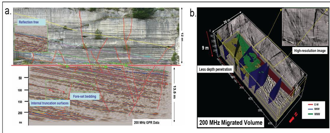
Figure 2: a). Quarry wall with fractures and bedding surface traced into the subsurface in the 100MHz GPR volume. b). 200 MHz migrated volume with stratigraphic and fracture interpretations.
