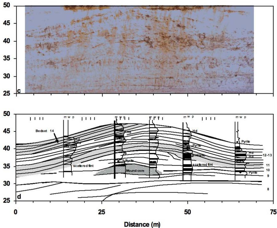
Figure 2: Photograph and line drawing of mound in the Faxø quarry, displaying the internal architecture of the deep-water coral reef.
