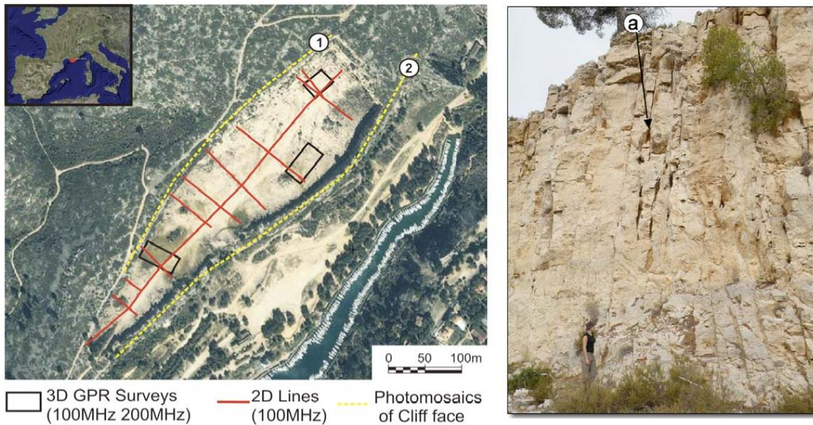
*Figure 1: Left: Map of Cassis Quarry: The quarry is over 500 m long and approximately 100 m wide, allowing for the examination of production scale lateral variability of the fracture network. The location of the 2D and 3D GPR data acquired in 2008 is shown. LIDAR scans of the cliff faces adjacent to the Quarry floor will be acquired in 2009. Right: Near vertical fractures in the quarry wall. Marker a shows how some of the fractures are solution enhanced .*
