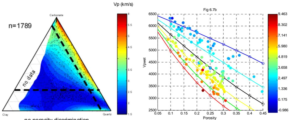
Figure 1: Example ternary diagram showing the relationships between P-wave velocity and textural and mineralogical composition (from Kenter et al. 2007) (left); Cross plot of porosity vs. P-wave velocity with the gammaK parameter from Sun's Extended Biot Theory superimposed. The gammaK parameter captures the frame flexibility at a given porosity and provides a mean to relate the pore structure of carbonate rocks to acoustic velocity variations (Weger et al. In press).
