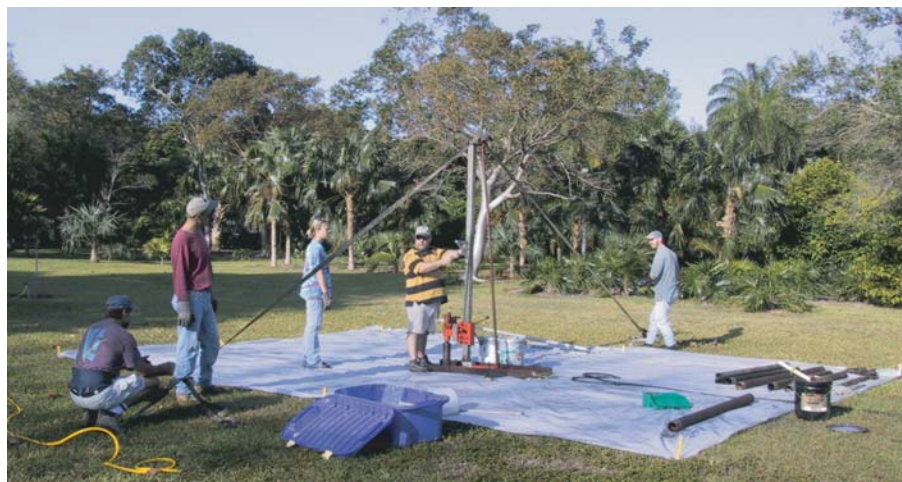
Drilling team working to get a core from the Miami Oolite that would be used for ground-truthing the GPR data and laboratory measurements.
