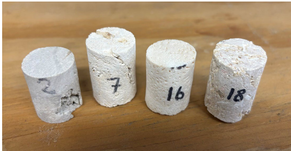
Figure 1: Examples of representative 1-inch core plugs from ES-103 illustrating the complexity of rock types in the different reef facies, and the challenges they represent for measuring acoustic velocity and resistivity.
